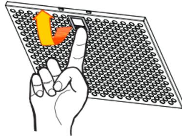
**Instruction:** To remove the filters, press the clip located at the front, pull down the filters, and release the clip.
